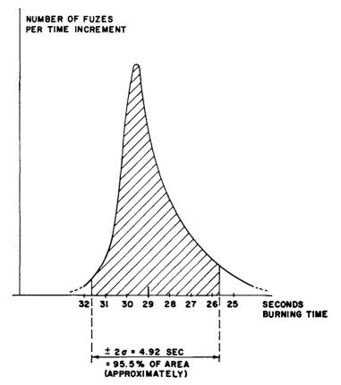
Fig. 4 Moderately Skewed Distribution of Delay Times for a Fuze Production
