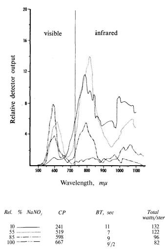
Fig. 2 Influence of Alkali on Radiant Energy Distribution
