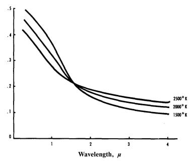
Fig. 1 Spectral Emissivity of a Typical Refractory Metal
