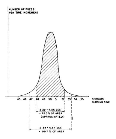
Fig. 3 Nearly Normal Distribution of Delay Times for a Fuze Production
