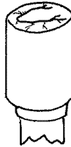
3. OUTER 40# ROLLED OVER CHIPBOARD AND CLOSED WITH TONGUE FOLD
