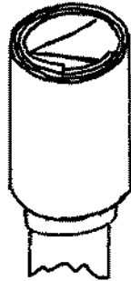
2. CHIPBOARD ROLLED OVER INNER BAG TO DIAMETER OF 1 3/4"
