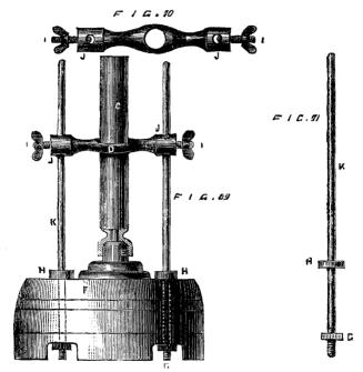
Fig. 69. c, gerb case; d, metal band to support the case; ii, supports for band, with hole for steel rods, klk; h, base of rod, resting on the upper part of lower part of rod, with nut and thread to fasten them to the block; dotted lines showing the lower part passing through the block; ii, thumb screws for fixing the block; e and f, block and nipple. Fig. 70. Band removed from the upright. Fig. 71. Rods (or uprights) removed from the band and block.
