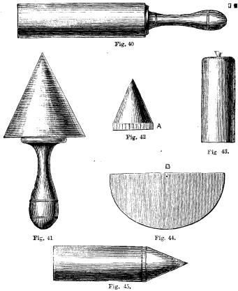
pot unoccupied for that distance; then take the upper part of the paper and turn it over the end of the former, and stamp it down on the workbench board, so as to close the end, Fig. 43; this when dry is ready for the cone. These are also made out of thin cartridge or brown paper, for the arge rockets,
