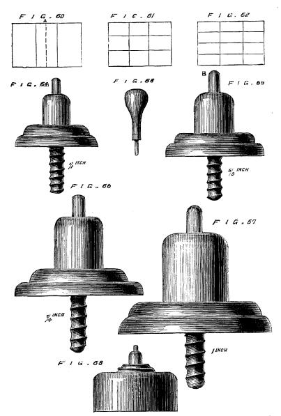
Fig. 60. Diagram of paper for 2oz. gerb, and 1oz. brilliant fire cases. Fig. 61. Diagram of board for 2oz. gerb cases. Fig. 62. Diagram of board for 1oz. brilliant cases. Fig. 63. Priming tool. Fig. 64. 1oz. nipple. Fig. 65. 2oz. nipple. Fig. 66. 2lb. nipple. Fig. 67. 2lb. nipple. Fig. 68. Sketch of nipple attached to the block.
