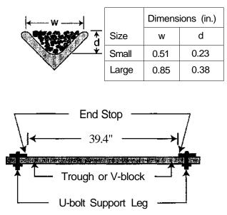
Figure 16-1. V-block made from a piece of angle iron.
