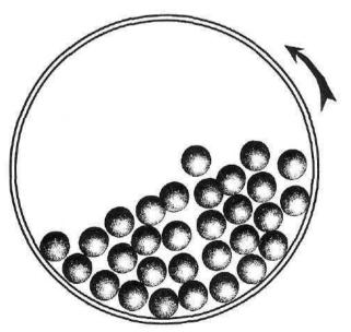
Figure 9-3. Start of cascading action
