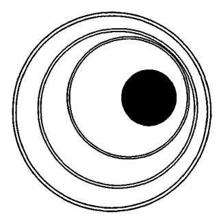
Figure 8-3. Ring and puck pulverizer rings
