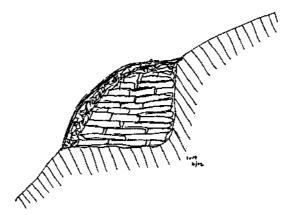
Figure 5-2. Charcoal Earth Kiln on Sloping Ground
