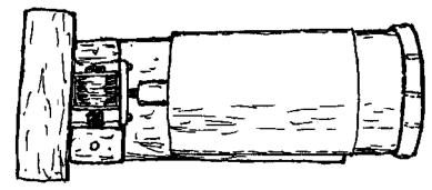
Figure 11-2. Ball mill - top view
