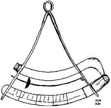
Figure 15-10. V-spring eprouvette
