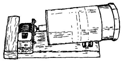
Figure 11-1. Ball mill - side view
