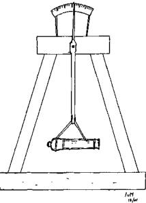
Figure 15-19. Basic ballistic pendulum
