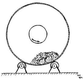
Figure 13-1. Du Pont's rod mill
