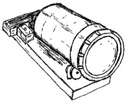
Figure 11-4. Ball mill - front view
