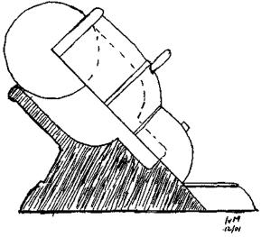
Figure 15-15. Mortar eprouvette cutaway view
