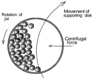
Figure 9-1. Motion of planetary ball mill
