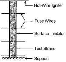
Figure 16-2. A strand used for testing
