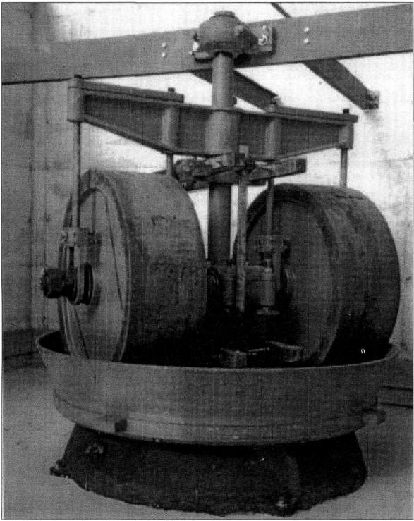
Figure 8-2. A wheel mill used in a modem Black Powder plant.
