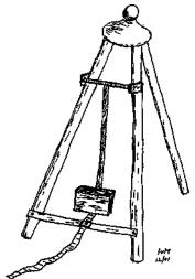
Figure 15-20. Ballistic target pendulum
