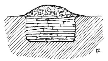
Figure 5-1. Charcoal Earth kiln on level ground
