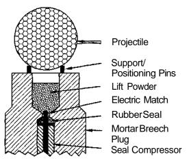
Figure 16-5. Cross sectional drawing of breech plug
