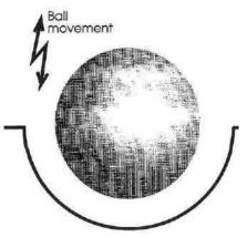
Figure 9-2. Vibratory ball mill mechanism
