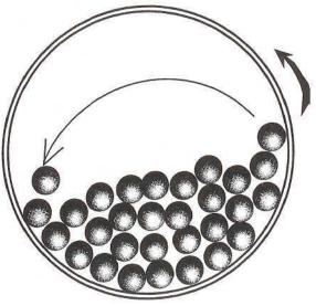
Figure 9-4, Action at critical point
