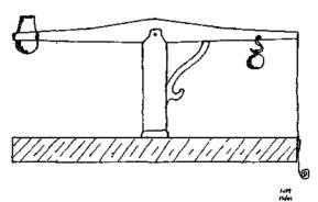
Figure 15-18. Du Pont's recoil gauge
