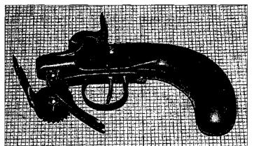
Figure 16-8. A working replica of a pistol eprouvette
