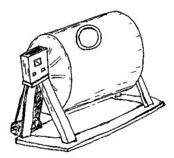
Figure 8-1. A small industrial ball mill
